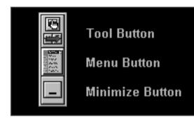
The Tool Button opens and closes My-T-Pen Control Panel in the normal / Supervisor Mode. In Operator Mode, the Tool Button does not function.
